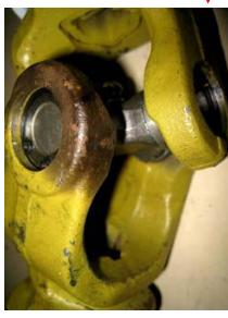
Typical cross failure due to blocked internal grease port
