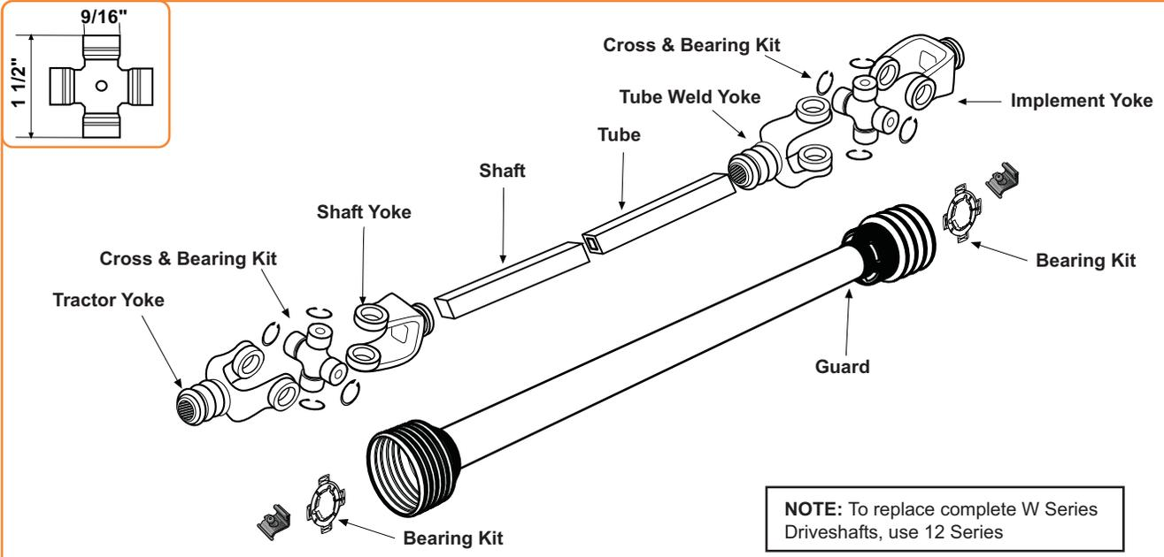
**NOTE:** To replace complete W Series Driveshafts, use 12 Series
