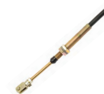
Cable - PTO (Proportional Drive 4WD) Length: 2340mm
